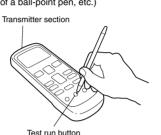
• To end test operation, press the remote control unit START/STOP button. (When the air conditioner is run by pressing the test run button, the OPERATION indicator lamp and TIMER indicator lamp will simultane-
