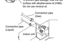
(3) When the flare nut is tightened properly by your hand, use a torque wrench to finally tighten it
