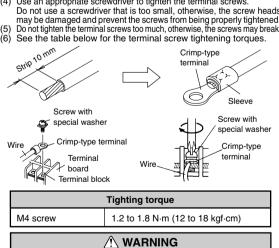
Use crimp-type terminals and tighten the terminal screws to the specified torques, otherwise, abnor-
