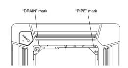
\* Align the stamped marks on the decoration panel against the pipe and the drain
