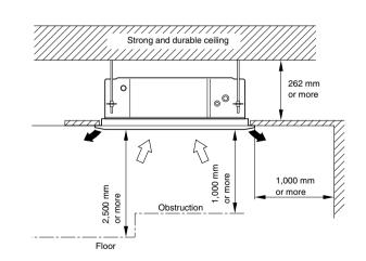
This product can be installed at a height of up to 3.5 m. Perform the Function Setting on the remote control in accordance with the installed height.
