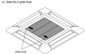
(2) Open the intake grille and remove.
